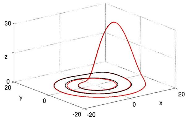
FIG. 4. (Color online) Plot of the two attractors:  $\mathbf{v}_1$  and  $\mathbf{v}_2$  in the case of  $\epsilon=0.07$  and  $\theta=0.15$ . The two curves nearly coincide and chaos has disappeared due to the particular coupling between the two chaotic oscillators.
