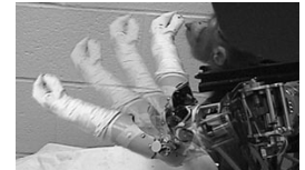
Image 4: A monkey feeds itself during a three-dimensional brain control task. In this experiment the monkey controlled the velocity of the arm's endpoint. In subsequent experiments, the monkey also controlled the opening and closing of the arm's grip (© The Dana Foundation)
