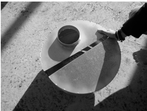
Figure 7. Image of the transition piece between the tube of plate and the top of the MGP
