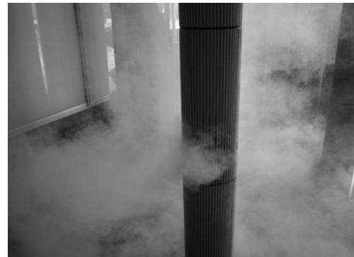
Figure 5. Tracer gas test in one of the MGPs during the implementation of the system, and how the air is distributed homogeneously at the outflow
