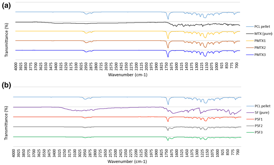
Fig. 5 Comparison of the FTIR spectrum of the PCL pellet and the pure drug with the drug-loaded scaffolds: a PCL pellet and pure MTX; b MTX-loaded scaffolds; c PCL pellet and pure 5F and d 5F-loaded scaffolds
