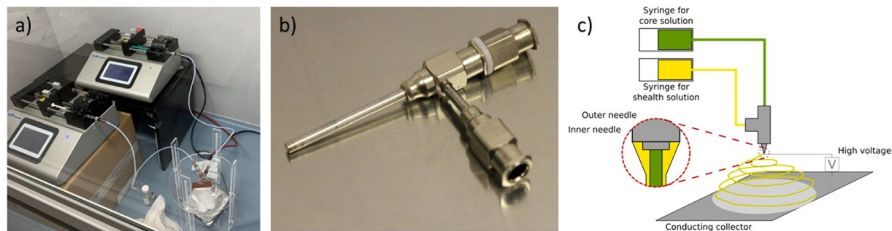
Fig. 1 a) Coaxial electrospinning set-up; b) coaxial nozzle of Ramé-Hart Instrument Co; c) schematic of the coaxial electrospinning process
