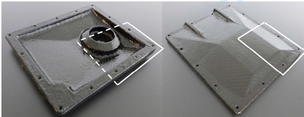
54 Figure 7 New oil sump after the lay-up process with carbon fibre 55 56 57 58 59 60
