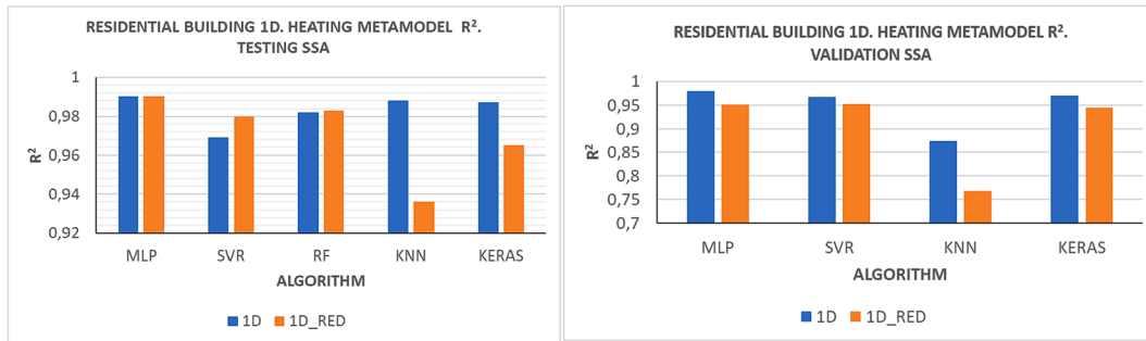
Fig. 8. Residential building 1D. Heating metamodels R^2 . Testing dataset (left) and validation dataset (right). SSA prediction.
