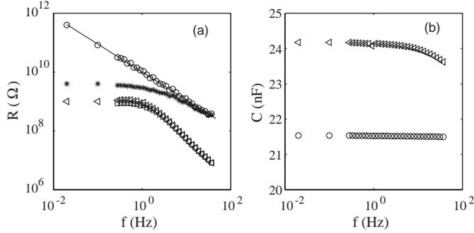
Fig. 1 – (a) Polycarbonate resistance  $R$  as a function of frequency measured at  $T_i = 433$  K ( $\triangleleft$ ) and at  $T_f = 333$  K ( $\circ$ ). The effect of the  $4\text{G}\Omega$  input resistance is also shown at  $T = 433$  K ( $\square$ ) and at  $T = 333$  K ( $*$ ). b) Polycarbonate capacitance *vs.* frequency measured at  $T_i = 433$  K ( $\triangleleft$ ) and at  $T_f = 333$  K ( $\circ$ ).
