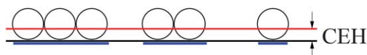
Fig. 4 Sketch for the meaning of the compact equivalent height (CEH) of a deposit.
