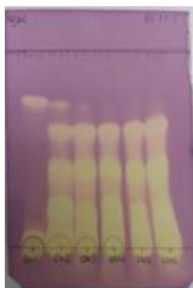
Figure 31. TLC (mobile phase: ethyl acetate–methanol–water (65:15:5 v/v/v)) of the six extracts post–sprayed with DPPH• solution to detect qualitative antioxidant in vitro activity. The yellow spots correspond to the positive result of the antioxidant activity against the DPPH free radical.
