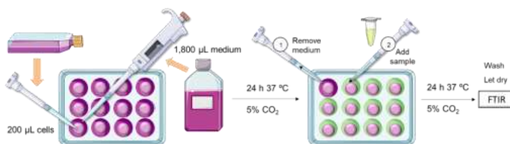
Figure 90. Scheme of FTIR method in cells: the cells were grown on a glass surface at 37 °C and 5 % CO 2 for 24 h. Then, the medium was replaced by sample at different concentrations in fresh medium and incubated for 24 h. Molecular changes in the cells were determined by FTIR analysis after washing and cleaning the glass containing cells.
