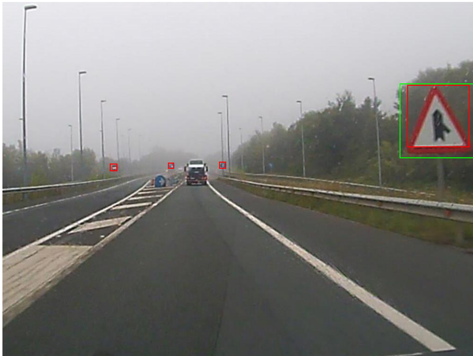
Figure 3-9. Example of false-negative detections due to the small size of the traffic sign. Table 3-4 shows detailed information.
