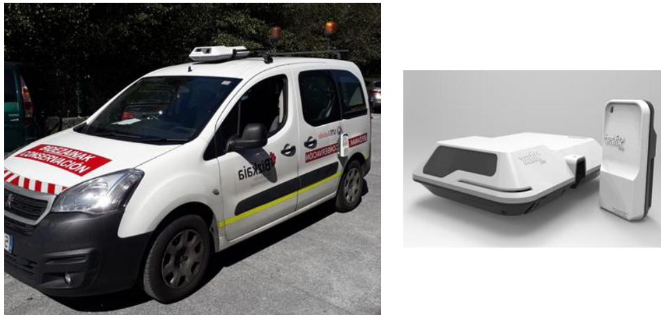
Figure 1-7. Data acquisition system installed in a road maintenance vehicle of Provincial Council of Bizkaia and managed by Gertek.
