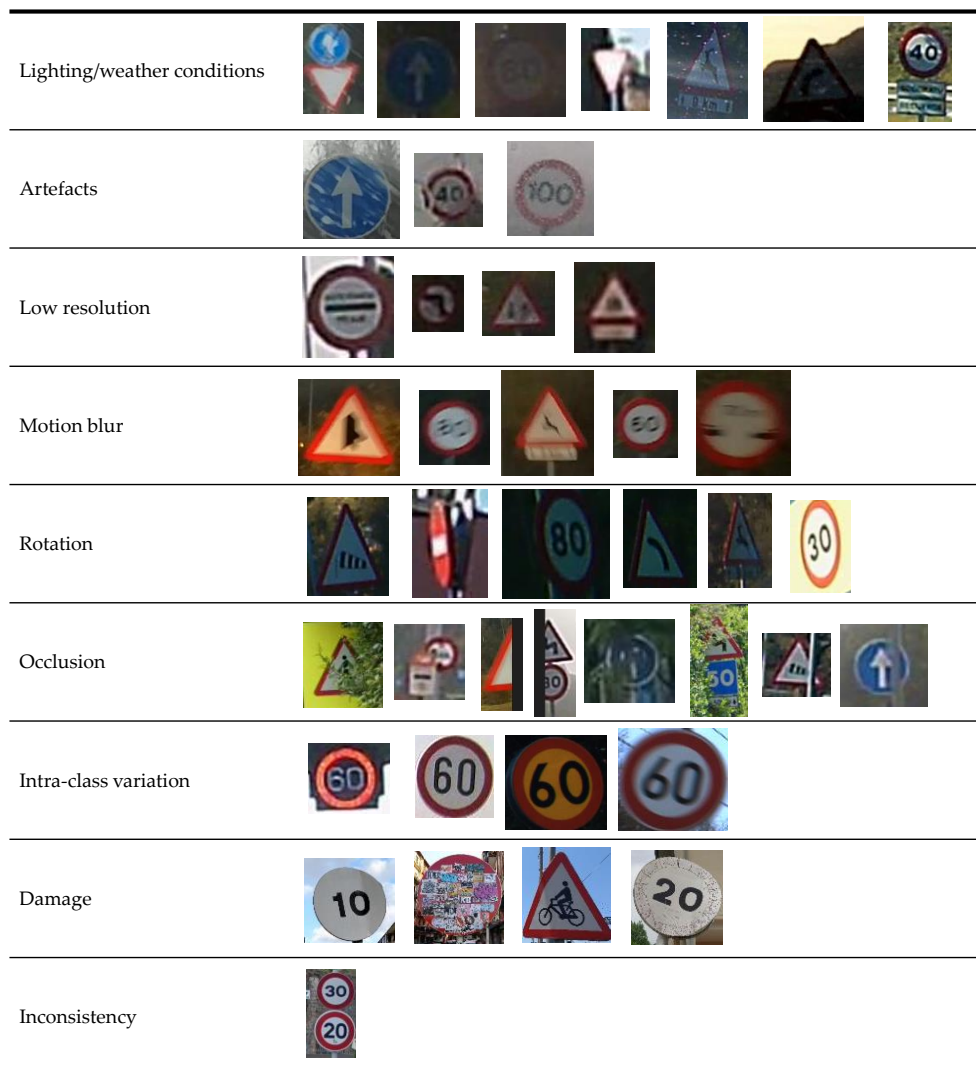
Figure 3-1. Sample images for TSR challenges: lighting or weather conditions, artefacts, low-resolution signs, motion blur, rotation, occlusion, damage, inconsistencies and intra-class variation (The vast majority of the samples are extracted from Ceit-TSR dataset).
