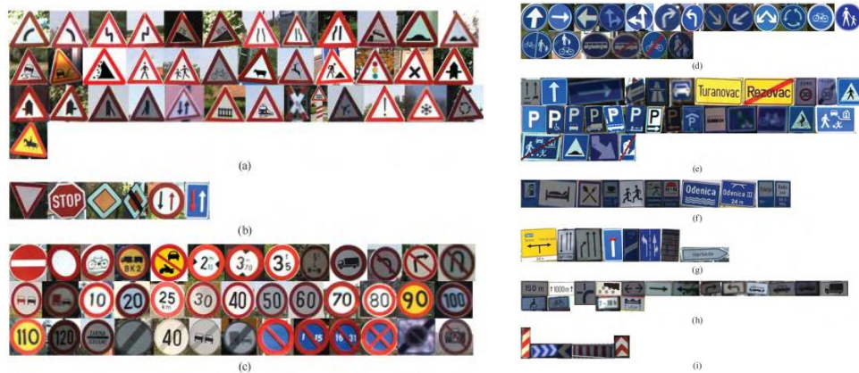
Figure 3-6. Traffic sign samples of the ETSDB dataset. There are 164 different classes grouped into 9 categories: danger, regulatory (priority, prohibitory, mandatory and special regulation) informative (information, direction and additional panels) and others.
