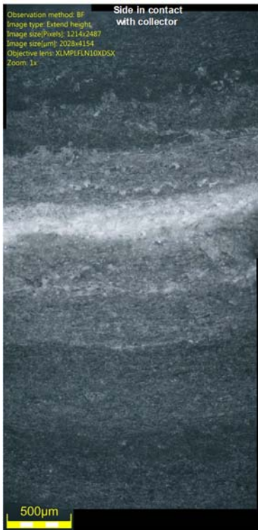
Figure 3. Optical image of the cross section surface in a sample of thirteen layers PVDF based material.
