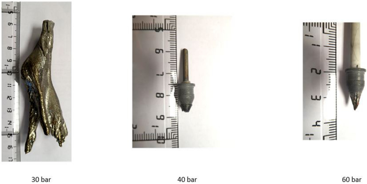
Fig. 18. Atomisations blocked due to Fe freeze around the melt nozzle, conducted at different inlet He pressures ( \Delta P = 0.25 bar, throat width = 0.6L_0 and \Delta T = 165^\circ\text{C} ).
